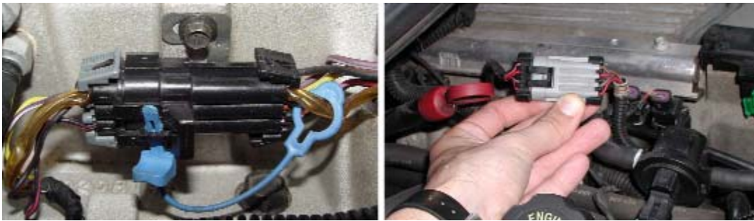
Figure 1: Opti-Spark Diagnostic Connectors - 1992 (left) and 1993-1996 (right)
