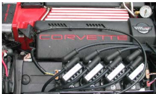
Figure 7: Proper Orientation of Ignition Wires
